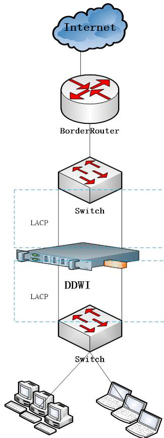
**FIGURE 2-6.** Transparent Bridge mode with LACP
